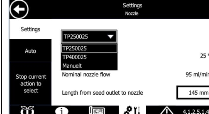
It is also possible to select the “manual” function in the nozzle, where is possible to customize the spraying angle and volume.
