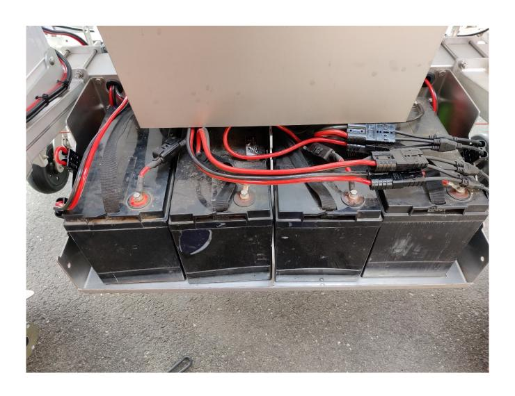
Please, when mounting the battery pack to AGM equipped robots, please remember to change the "BATTERY DISCHARGED SET" value to 23V.
