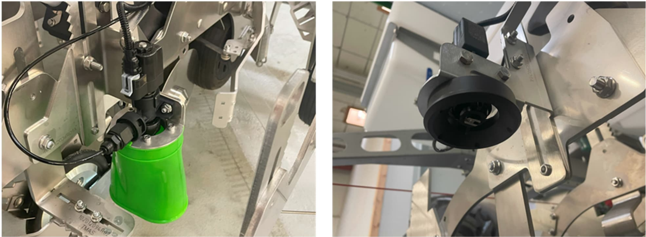
Figure 4 - nozzles with and without the wind-drift cover
